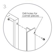
3. Thanks to the multifunctional T-shaped posts, all kinds of shapes can be created with the panels. The panels can be installed on ground level thanks to the long anchoring pins at the bottom of the T-shaped posts.
